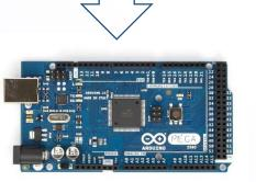
Processing Unit: Arduino MEGA (Microcontroller)
