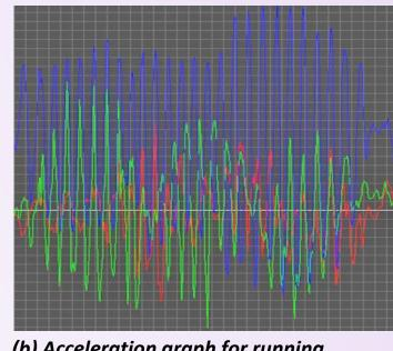
(b) Acceleration graph for running Red – y component; Green – x component; Blue – z component
