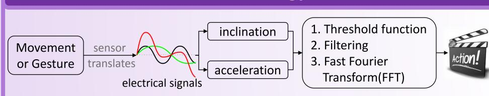
The sensor should correspond to our balance system, so it was placed close to the ear in fixed orientation. It translates the detected movements into electrical signals for further analysis:
